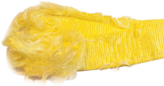
TENSION BREAK LOOSE THREAD
